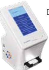
Eurofins Technologies offers a quick and easy-to-use protein-based testing method to identify genetically-modified raw ingredients like corn, soybean and canola before they are processed into a final product. The RapidScan reader provides an easy and on-site quantitative interpretation of the results in only 10 minutes.
