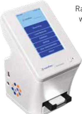
RapidScan is unique to the market for multiple allergen testing, and compatible with Eurofins Technologies' wide range of allergen lateral flow devices. The reader is easy to set up and operate, generating quantitative results within a few minutes. Data can be stored on the reader then exported through a USB port.
